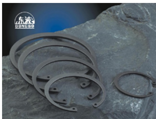
DIN6799 / D1500/RA Material: Steel, Stainless Steel Size: 0.8mm-30mm Surface: Black, Phosphated, Zinc Plated
