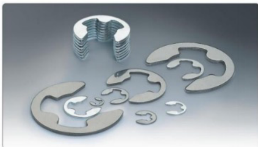
DIN6799 / D1500/RA Material: Steel, Stainless Steel Size: 0.8mm-30mm Surface: Black, Phosphated, Zinc Plated
